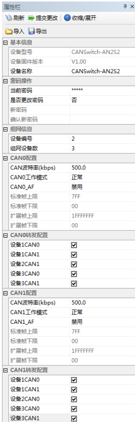
Figure 3.6 Configuration of the second CANSwitch
