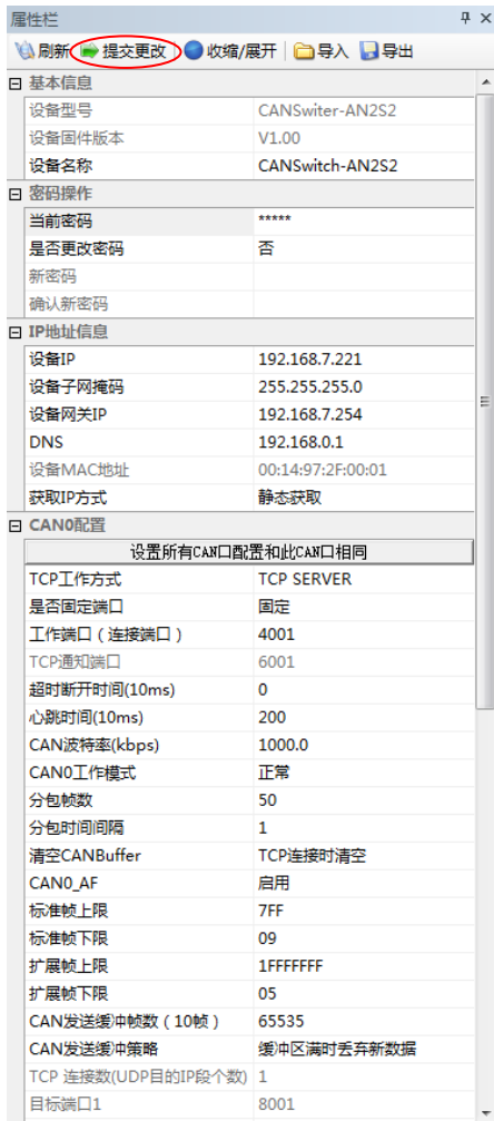
Figure 4.13 Configuration in TCP Sever mode
