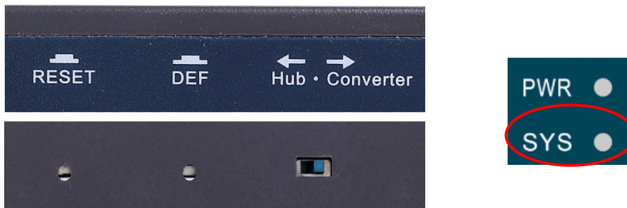
Figure 2.6 Reset button, default restoration button and function switch
