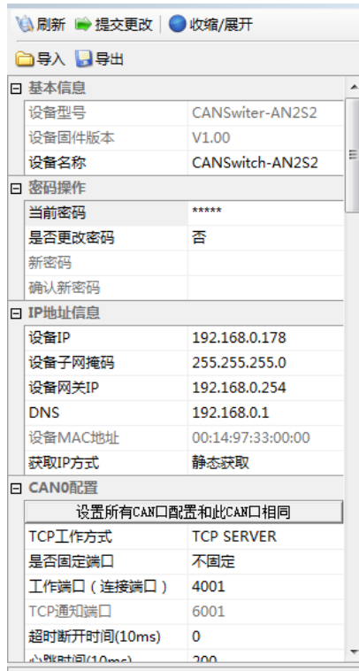
Figure 5.13 Modifying CANSwitch-AN2S2 device configuration properties
