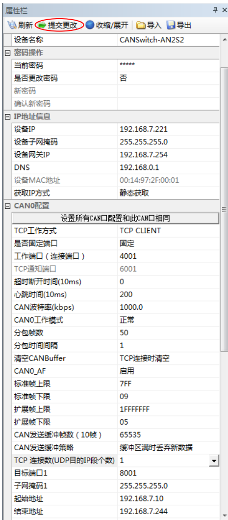
Figure 4.30 Configuration in TCP Clarinet mode
